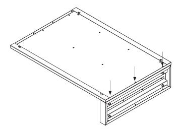
Attach the 2 insert compartments with 2 x 3 truss head screws.
